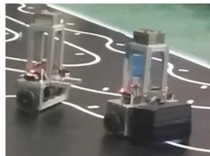
Fig. 1 Line tracking control performance by two balancing robots in the master-slave formation
